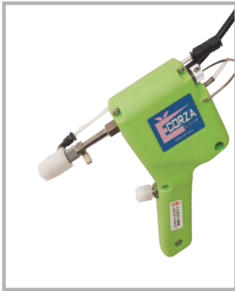
Drying air will come out from between nozzle head cover
